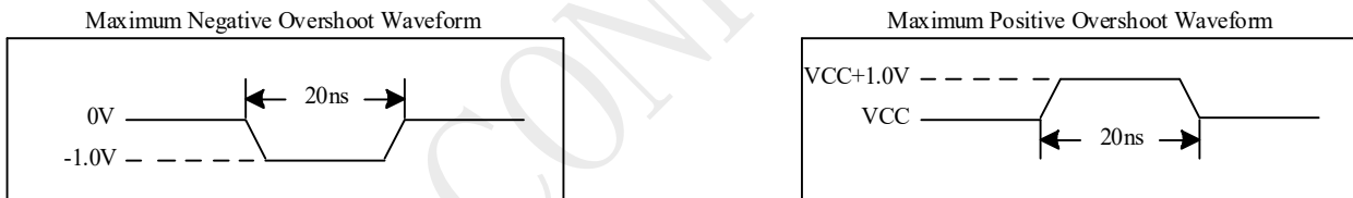
Figure 5-3 Maximum Overshoot Waveform
