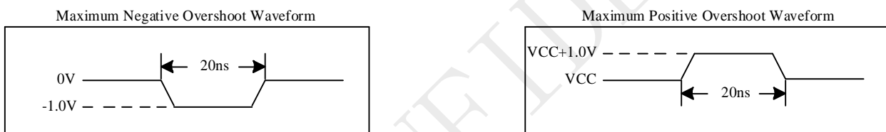
Figure 5-2 Input Test Waveforms and Measurement Level
