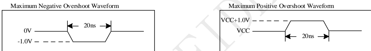
Figure 5-1 Maximum Overshoot Waveform
