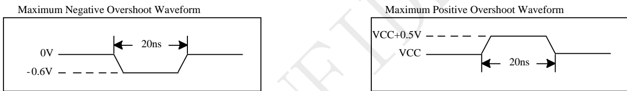
Figure 5-1 Maximum Overshoot Waveform
